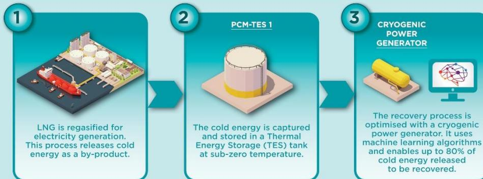
Cold energy recovered can be used for applications such as district cooling systems. This can be done by transporting the cold energy to another TES tank.
