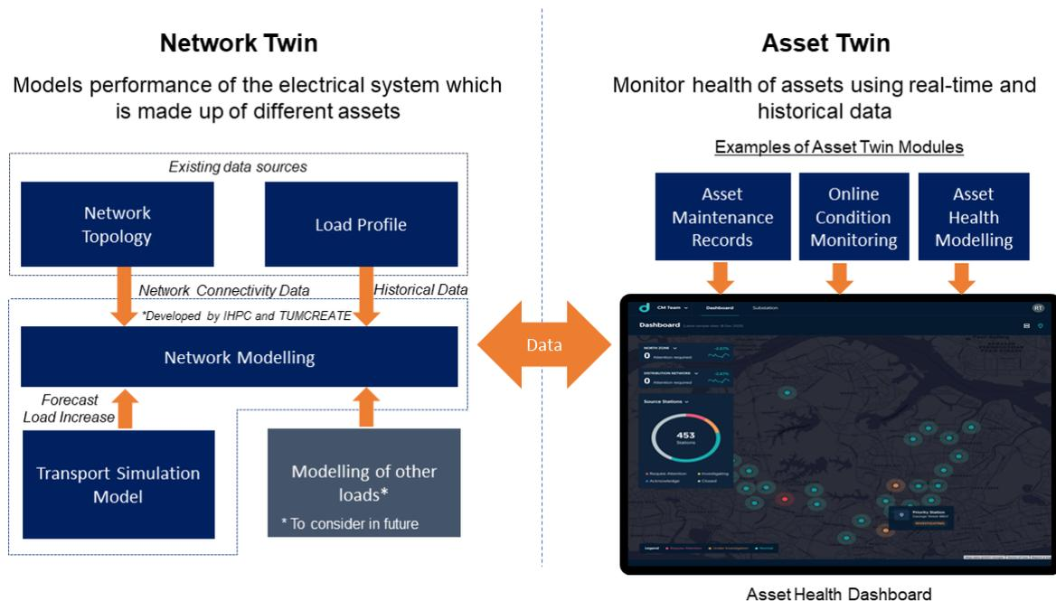
*Grid Digital Twin comprising the Asset Twin and Network Twin
