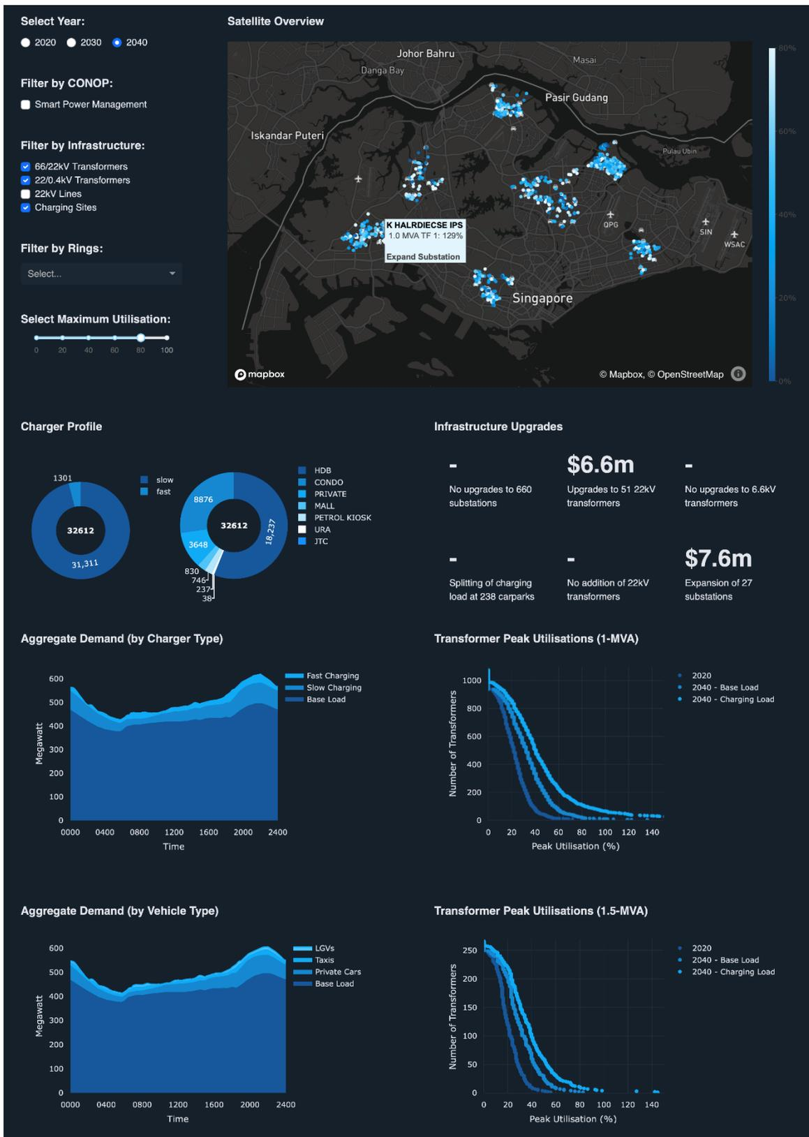
*Dashboard for analysing electric vehicle charging impact on the distribution grid using the Network Twin
