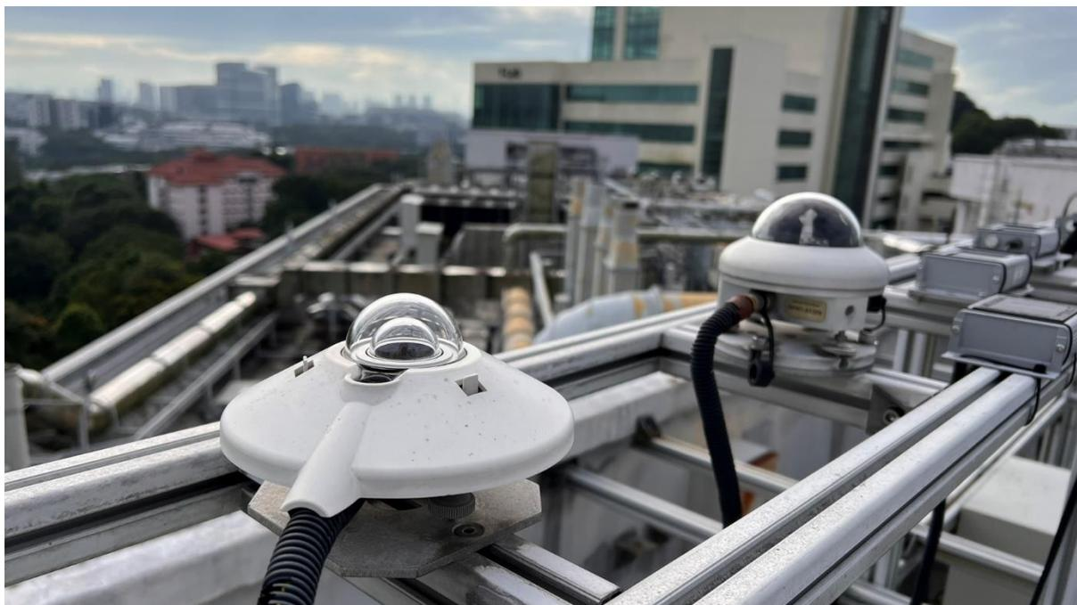
*A type of irradiance measurement instrument installed on building rooftops
