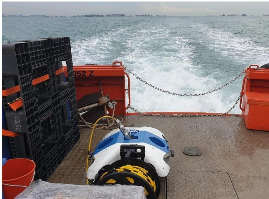
*Caption: Close-up view of BeeX Pte Ltd's existing Hovering Autonomous Underwater Vehicle (HAUV)
