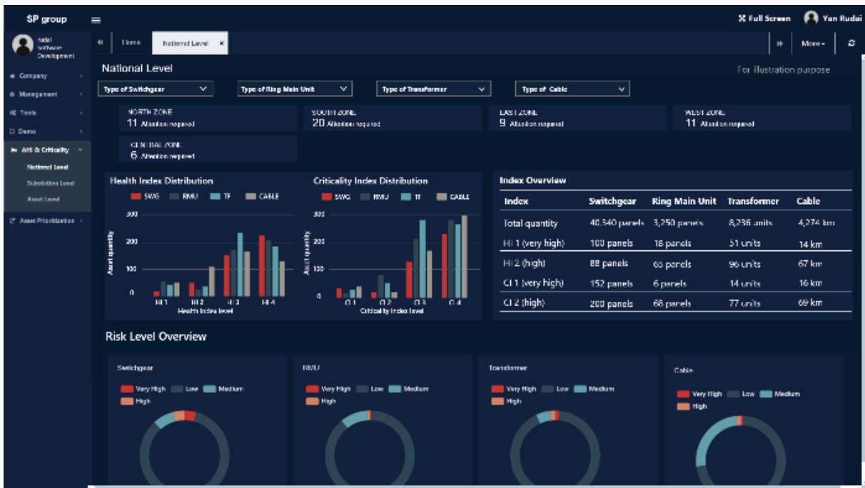
Overview of Asset Health and Criticality Index for the Distribution Network (Image Credit: SP Group-NTU Joint Laboratory)
